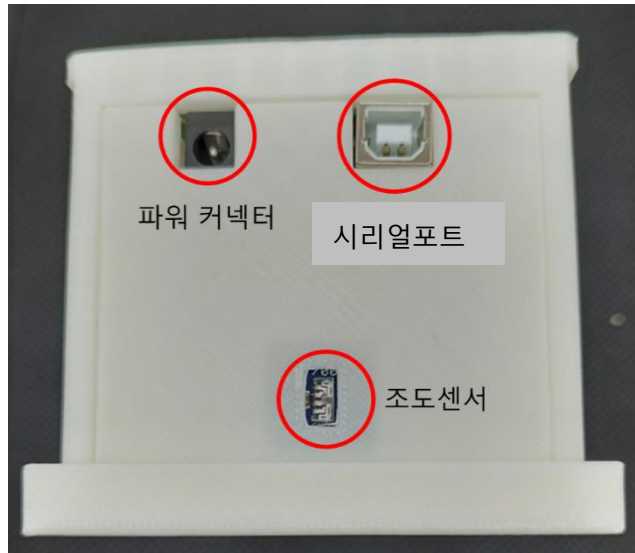
Figure 8. Top view of integrated sensor module
