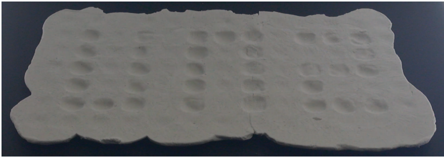
Figure 3.16: 'SNU' cells that are actuated can be (A) molded using gypsum to create an (B) 'SNU' mold.
