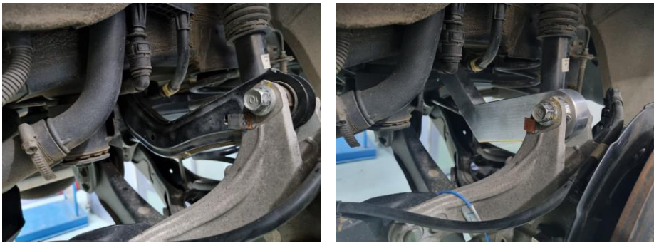
Figure 4.1 Target component of vehicle system (left) and the frame-shaped alternatives (right)
