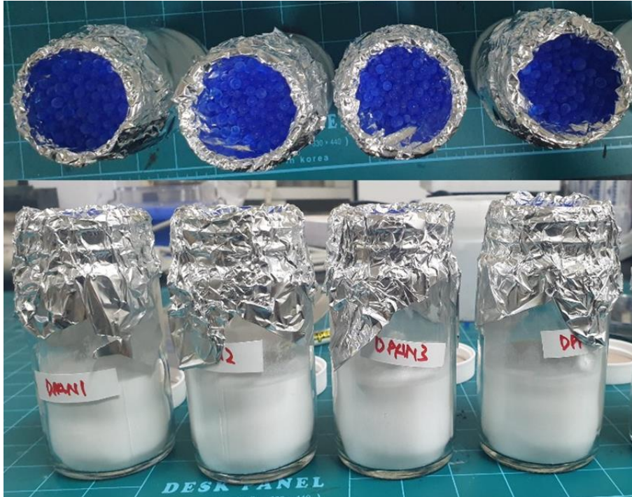
Figure 4-1. Photographs illustrating the drying process of PAN powder.
