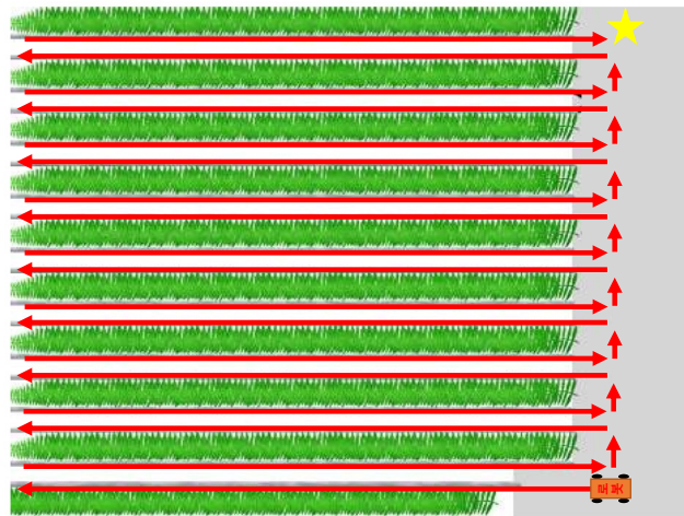
Fig. 2-20 Full path for greenhouse environment driving
