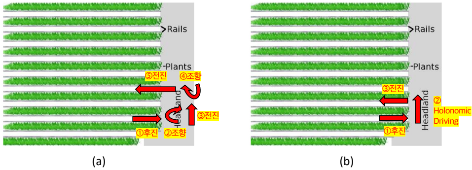
Fig. 2-4 How to enter the next working path according to wheel: (a) general robot wheels (b) mecanum wheels
