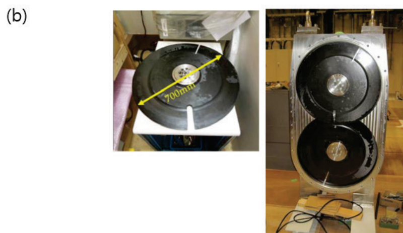
Figure 3.6 Details of the AMATERAS spectrometer. (a) Schematic view of AMATERAS. (b) Installed disc (left) and inside view (right) of the third fast disc chopper (used for monochromatisation) in AMATERAS [Ref. 3.17].
