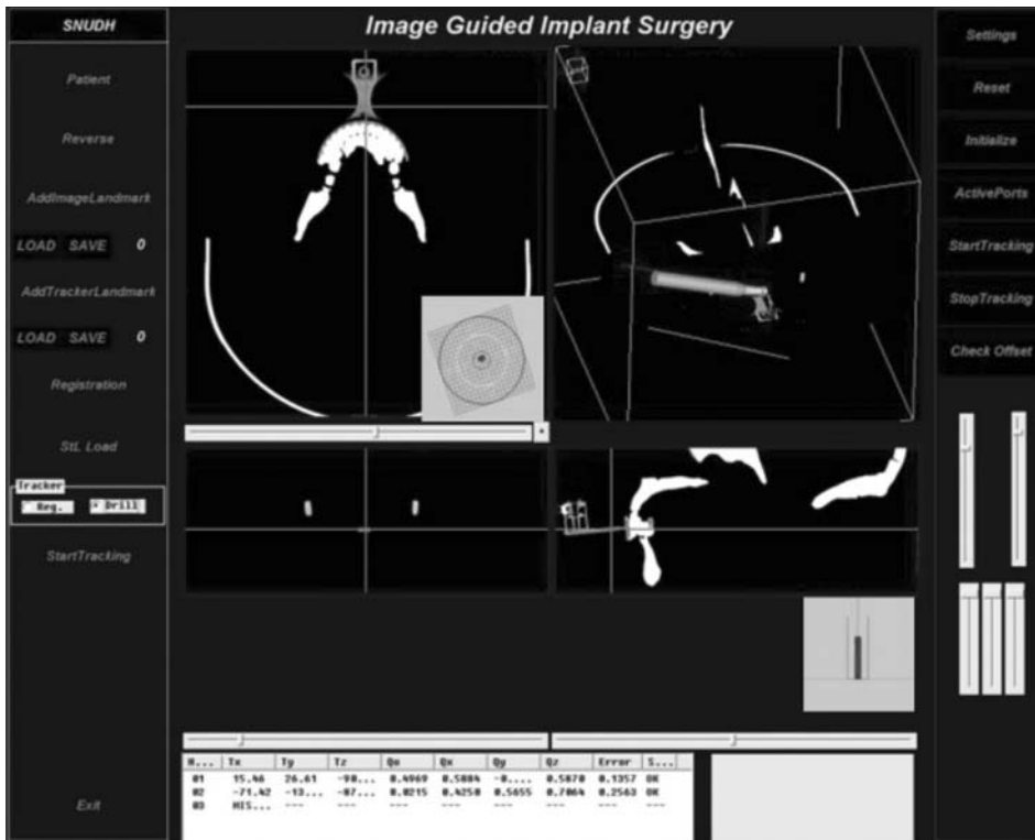
Fig. 2. Developed PC program for the image guided navigation system for oral and maxillofacial surgery providing information for position, angle and depth.
