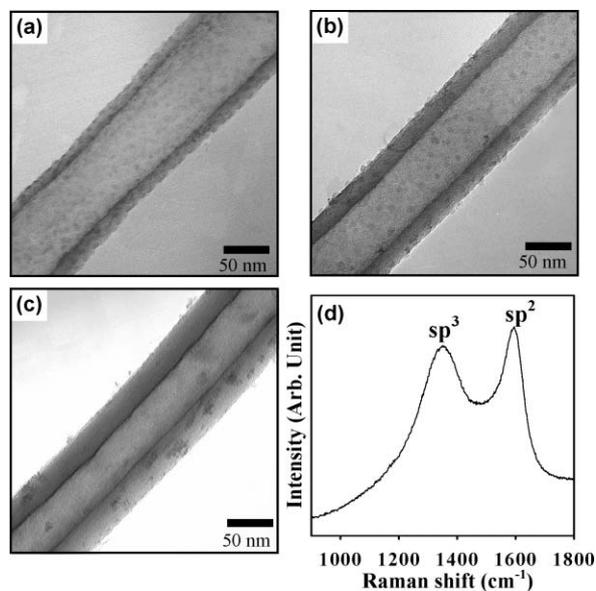
**Fig. 3** (a), (b), (c) TEM images and (d) Raman spectrum of the carbon nanotubes with tunable wall thickness originated from polyimide.
