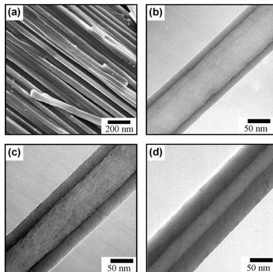
**Fig. 2** SEM image (a) of polyimide nanotubes prepared using AAO membranes and TEM images representing the wall thickness variation by controlling the concentration of polymer precursor solution: (b) 0.02 wt%, (c) 0.05 wt%, and (d) 0.1 wt%.
