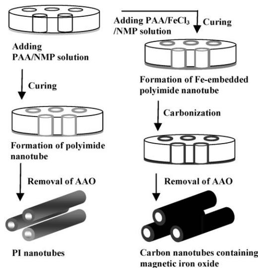
**Scheme 1** Schematic diagram of fabrication of PI nanotubes and carbon nanotubes containing iron oxide by wetting method using an AAO template.
