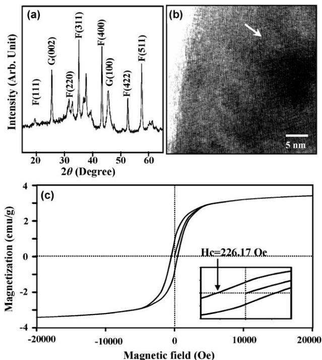
**Fig. 4** a) X-ray diffraction pattern, b) HRTEM image and c) hysteresis loop of  $\text{Fe}_2\text{O}_3$  embedded carbon nanotubes generated from polyimide nanotubes. The inset graph is hysteresis loop between  $-350$  and  $350$  Oe expanded.
