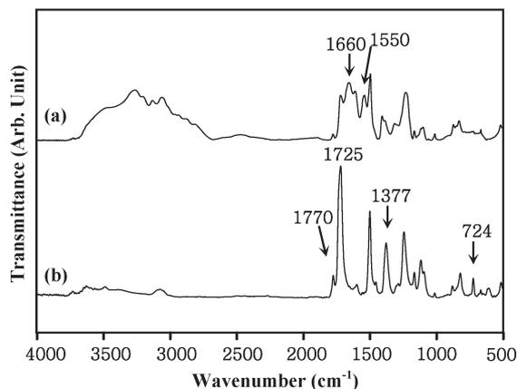
**Fig. 1** FT-IR spectra of (a) PMDA-ODA poly(amic acid) and (b) polyimide nanotubes in the channel of AAO membrane.
