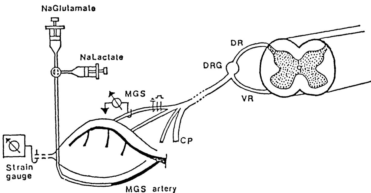
Fig. 1. A diagram of experimental set up. Medial gastrocnemius nerve (MGS) was stimulated electrically by platinum electrode. Achilles tendon was cut, tied to a silk and connected to force transducer. Various solutions were infused by sural artery.
