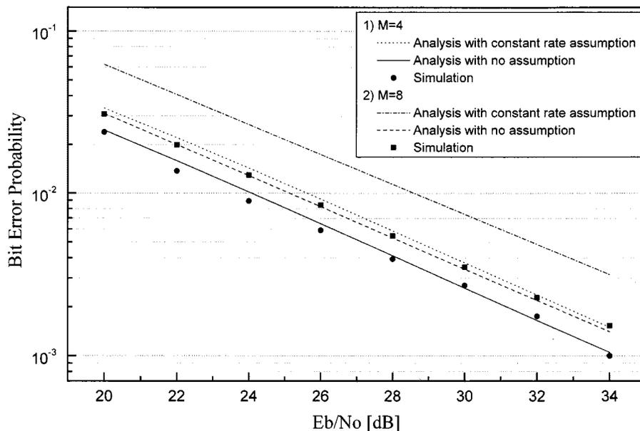
Fig. 3. Bit-error probability for  $M = 4, 8$ ,  $h = 2$ , and  $F_{DM}T = 0.025$ .
