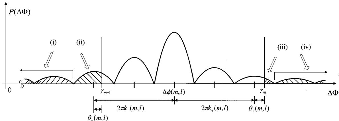
Fig. 2. PDF of LDI output with the parameters in (3).
