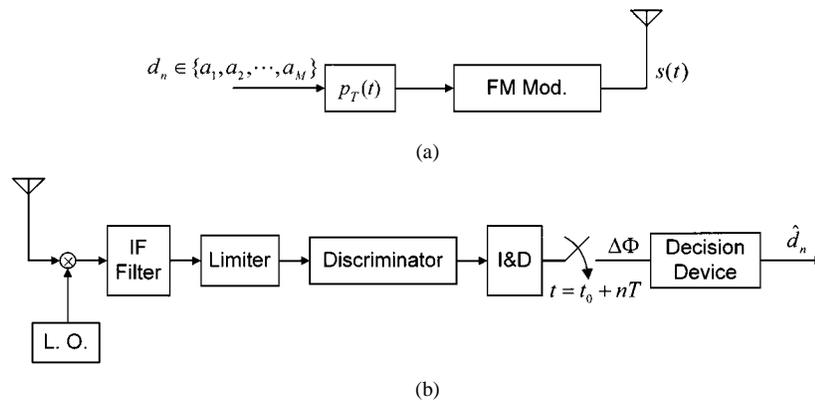
Fig. 1. System model. (a) Transmitter. (b) Receiver.
