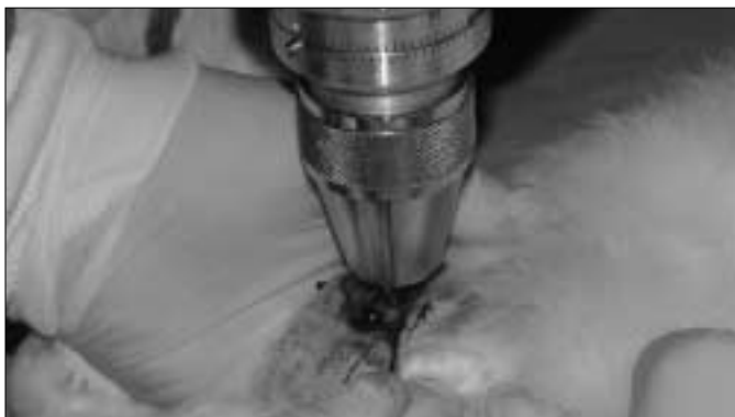
Fig. 2. A photograph of the removal torque tester holding the sample. The mount is connected to the implant and the jaws of the RT tester firmly grab the mount.
