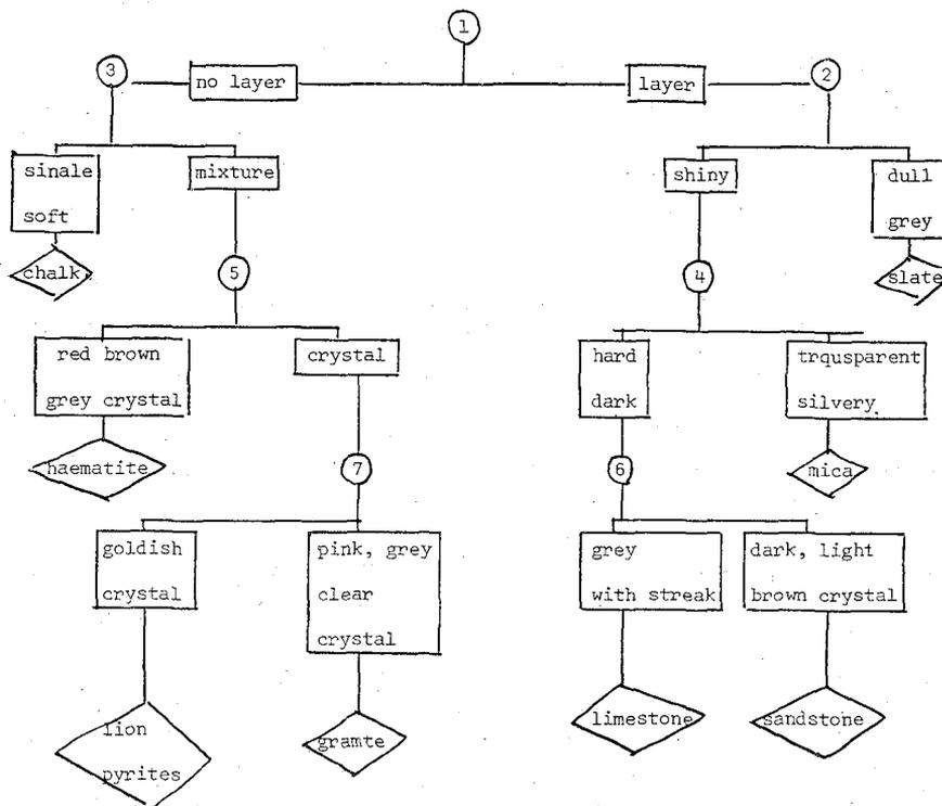
Fig. 3. The flow diagram according to the clues of the questions.
