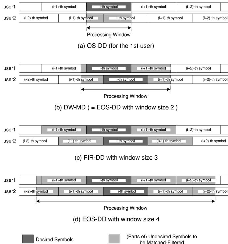
Fig. 1 Examples of OS-DD, DW-DD, FIR-DD and EOS-DD ( $K=2$  and  $L=1$ ).
