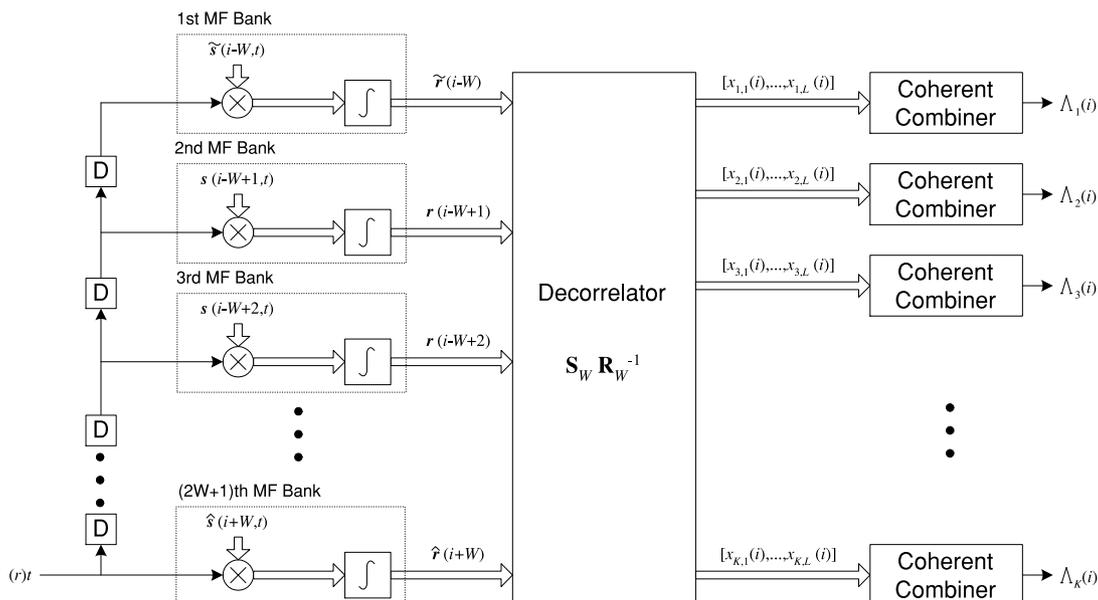
Fig. 2 Block diagram of the EOS-DD.
