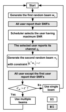
Fig.2: The procedure of (2x1) MUDAM scheme
