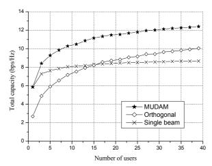
Fig. 3 The capacity in Rayleigh fading channel (SNR =20dB)
