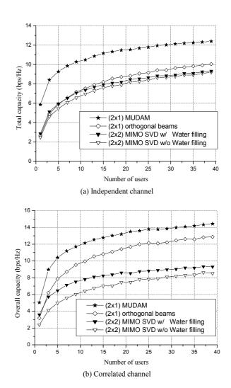
Fig. 4 The capacity of (2x1) MISO and (2x2) MIMO SVD
