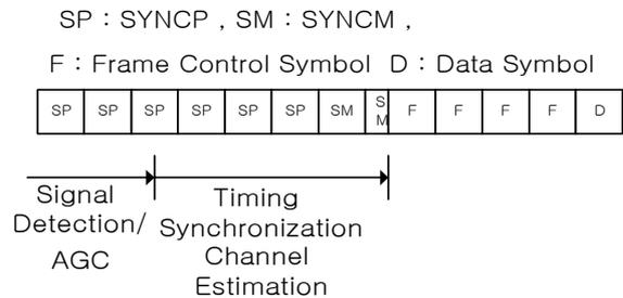
Fig. 1 Frame Structure for HomePlug 1.0
