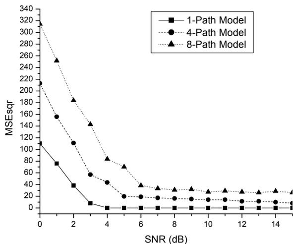
Fig. 6  $MSE_{sqr}$  for timing synchronization
