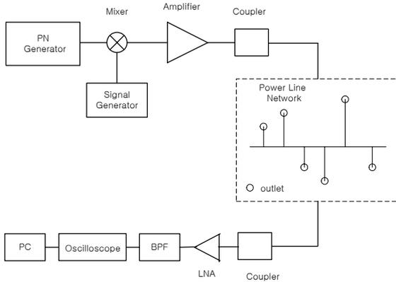
Fig. 2 Channel Sounding System
