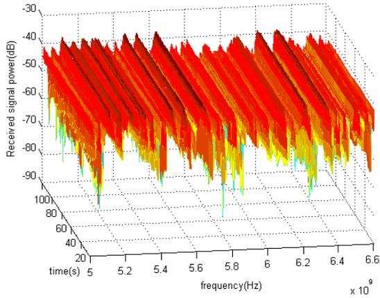
Figure 2. Measured channel transfer function at a LOS receiver position over 100 seconds
