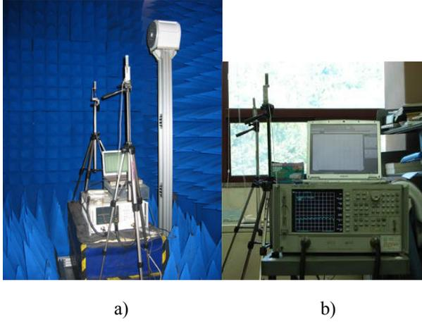
Figure 1. Measurement system in a) anechoic chamber and b) measurement environment
