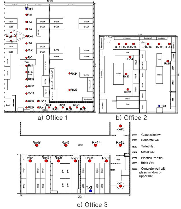
Figure 3. Ground plans and wall types of three offices where measurements performed
