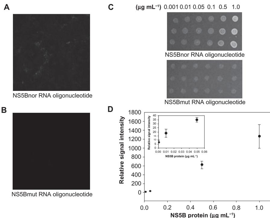
**Figure 5 A, B** Selective specificity of HCV-NS5B viral protein by QDs-conjugated RNA oligonucleotide. The NS5Bnor and NS5Bmut RNA oligonucleotides were bound on an immobilized viral protein chip, respectively. **C, D** Effect of HCV-NS5B viral protein concentrations on binding assay.
