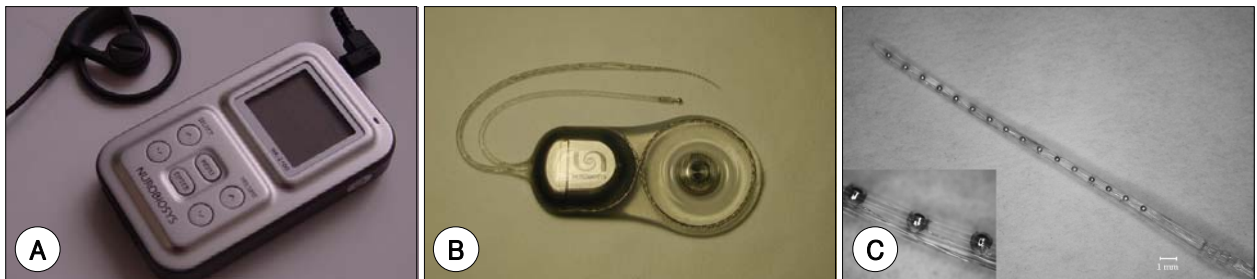
Fig. 1. A : Wearable-type Speech Processor of Neurobiosys cooperation. B : Receiver-stimulator implant of Neurobiosys cooperation C : Array of intracochlear electrodes of Neurobiosys cooperation.
