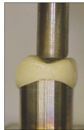
Fig. 3. Testing setup in the universal testing machine and position of load tip of test specimen and piston.
