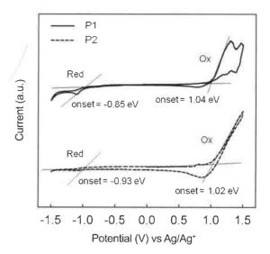
Figure 3. Cyclic voltammograms of P1 and P2.
