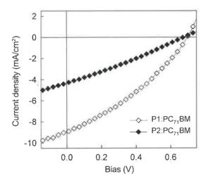
**Figure 8.** J-V curves of photovoltaic devices using  $PC_{71}BM$  as an electron acceptor.
