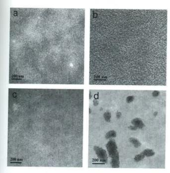
**Figure 6.** TEM images of **P1**:PC<sub>61</sub>BM blend films (a: asspun, b: annealed) and **P2**:PC<sub>61</sub>BM blend films (c: asspun, d: annealed).
