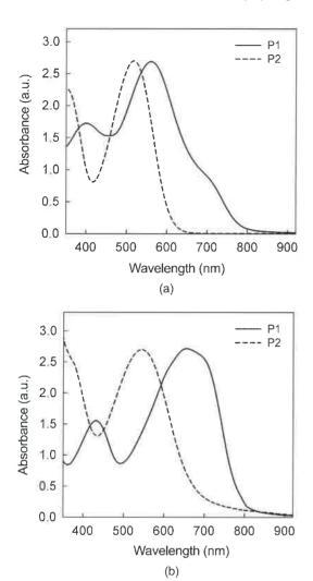
Figure 2. UV-Vis absorption spectra of the copolymers in chloroform solution (a) and solid state (b).
