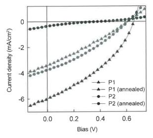
**Figure 5.** Current-voltage (J-V) characteristics of photovoltaic devices based on P1:PC<sub>61</sub>BM (1:4 w/w) (a) and P2:PC<sub>61</sub>BM (1:3 w/w) (b).
