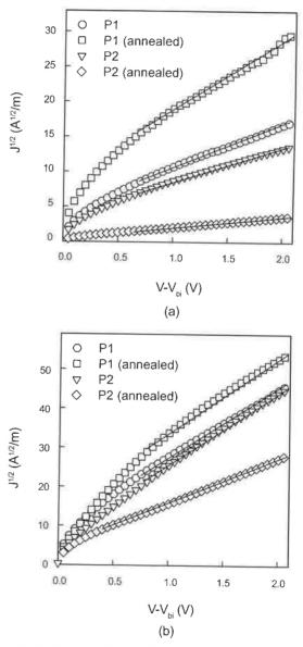
**Figure 7.** Dark J-V characteristics for hole-only (a) and electron-only (b) devices of  $P1:PC_{61}BM$  and  $P2:PC_{61}BM$ . The solid lines are the best linear fit of the data points.
