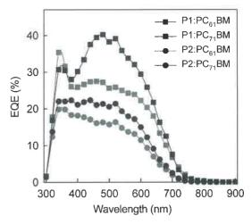
Figure 9. External quantum efficiency spectra of polymer/PCBM solar cells.
