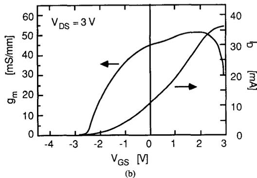
Fig. 3. (a)  $I$ - $V$  characteristic and (b)  $g_m$  curves of the integrated InGaAs JFET.
