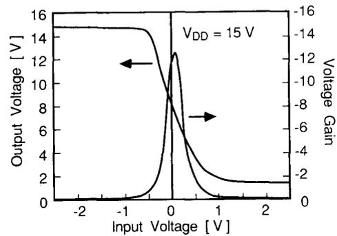
Fig. 4. DC voltage transfer curve and voltage gain of the preamplifier.
