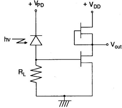
Fig. 2. Circuit diagram and photomicrograph of fabricated receiver OEIC chip. The chip has a size of  $500 \times 600\ \mu\text{m}^2$  and contains 1 p-i-n PD, 1 bias resistor, and 2 JFET's.
