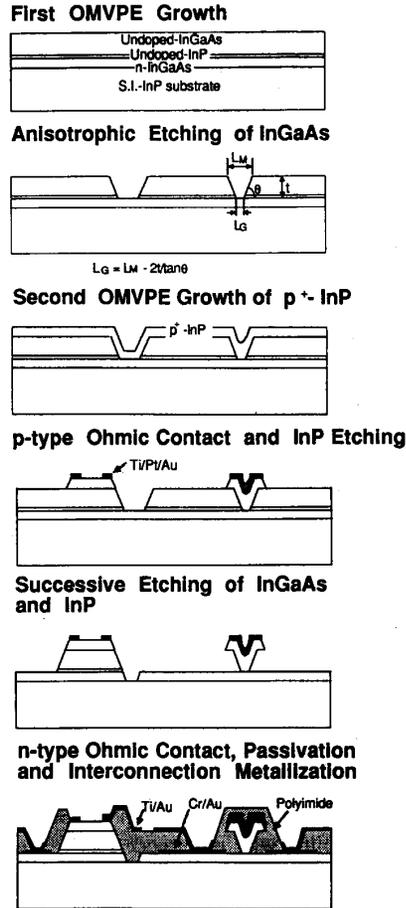
Fig. 1. Schematic cross-sectional views of receiver OEIC in fabrication steps. InGaAs p-i-n photodiode and self-aligned JFET are integrated on a S.I.-InP substrate.
