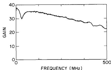
Fig. 4. Frequency response of a typical three-stage amplifier.
