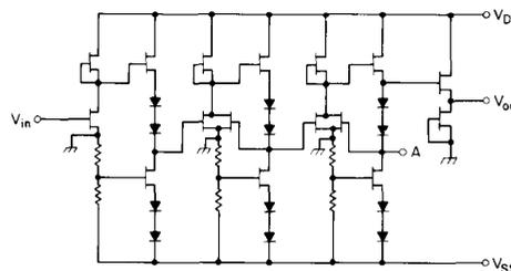
Fig. 2. Circuit diagram of three stage amplifier.
