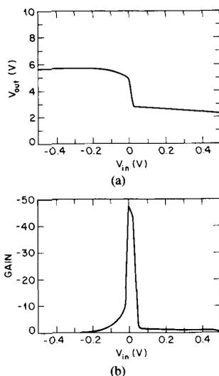
Fig. 3. DC characteristics of three-stage amplifier: (a) transfer characteristics and (b) gain calculated from transfer curve as a function of  $V_{in}$ .
