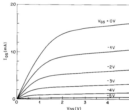
Fig. 1. Drain current-voltage characteristics of a typical InP JFET with a drain saturation current of 150 mA/mm.
