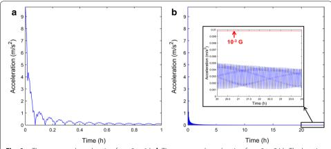
**Fig. 6** a Time-averaged acceleration from 0 to 1 h, b Time-averaged acceleration from 0 to 24 h. The location of analysis is  $[\Delta x \Delta y \Delta z] = [0.1 \text{ m } 0.1 \text{ m} 0.1 \text{ m}]$  from the center of the clinostat. The acceleration is smaller than  $10^{-3}$  G when reached 24 h
