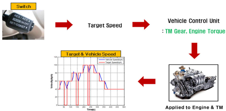
Figure 2.1 Operating Principle of Auto-cruise Vehicle Powertrain
