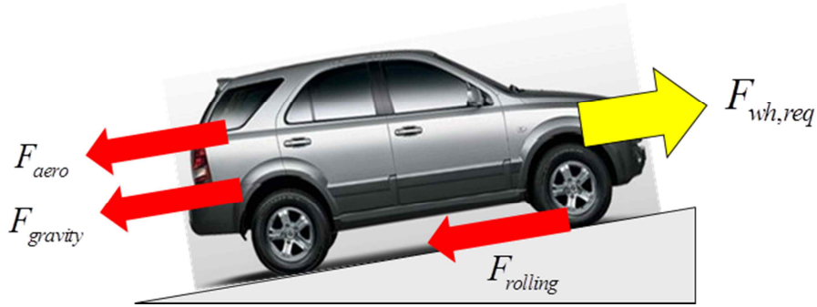
Figure 4.6 Traction and Load of Vehicle Dynamics
