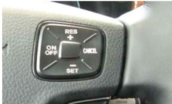
Figure 2.3 Switch Buttons of the Auto Cruise Vehicle
