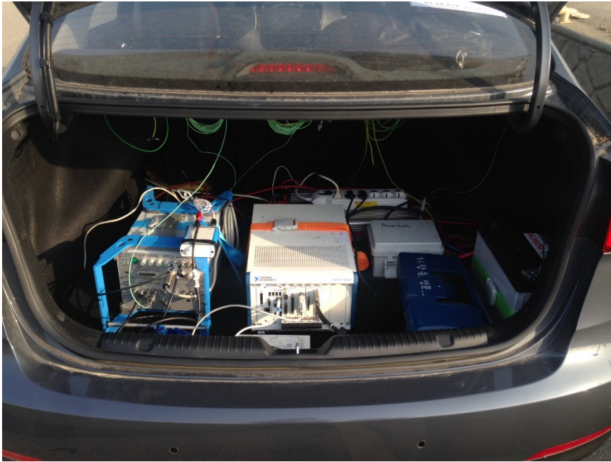
Figure 5.32 closed loop control system set up in test vehicle
