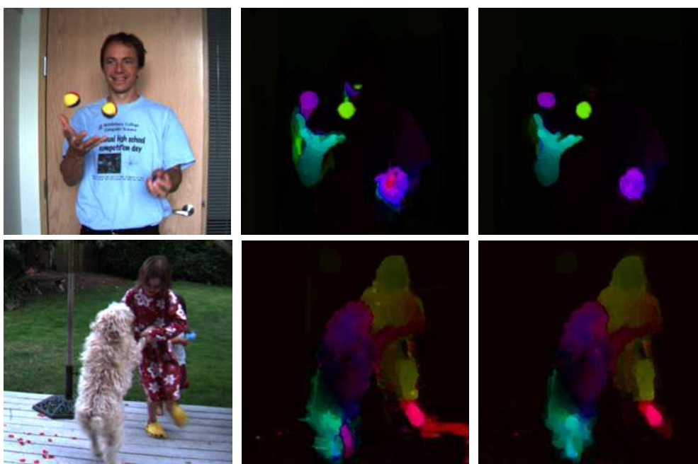
Figure 4.3: Flow estimation on the Middlebury test data set without the groundtruth flow (high-speed camera sequences.) Left column: The 10th frames in the Beanbag, the Dogdance Center column: Results from the bilateral kernel. Right column: Results from the proposed kernel. The proposed model shows better smoothing result inside motion segments while keeping sharp boundaries. The HSI color code is changed for better visualization of the difference.
