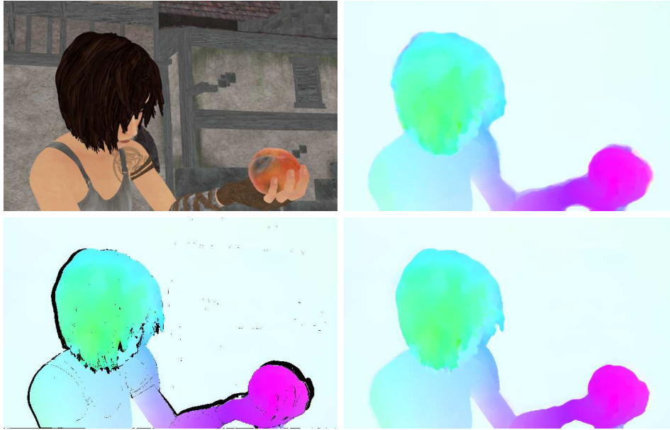
Figure 5.5: Estimation results for the Alley 1 sequence. Top left: The reference frame. Top right: Flow estimation with our method, which does not use occlusion detection. Bottom left/right: Flow estimation with our method. Detected occlusion is shown in black in the left image.
