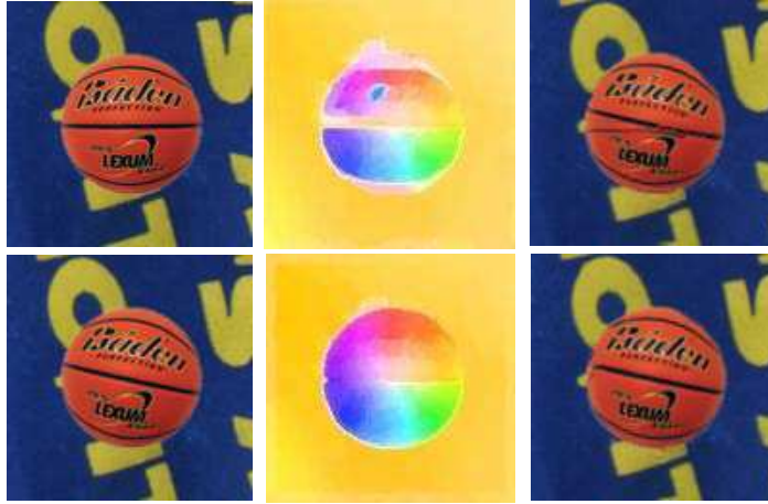
Figure 4.1: Flow estimation involving rotation. Left top and bottom: Input images with a rotating basketball synthesized on smoothly varying background (part of the Schefflera sequence.) Center and right top: Flow and deformed image from 11 \times 11 support window-based matching with 8-neighborhood prior. Center and right bottom: Flow and deformed image from the proposed model. The flow images are illustrated by the HSI color space (direction: hue, magnitude: saturation)
