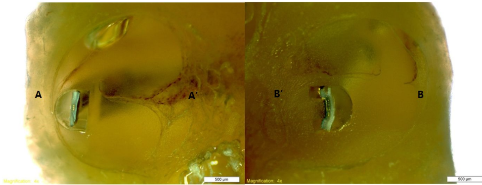
Figure 3.14 Cross-sectional View of the Human Cochlea with LCP-based Cochlear Electrode Array #5, Rupture of the basilar membrane is observed.
