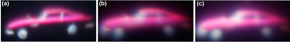
Figure 2.11 Comparison of the image blur of the Lamina 3D displays according to the number of layers: (a) three layers, (b) four layers, and (c) five layers.
