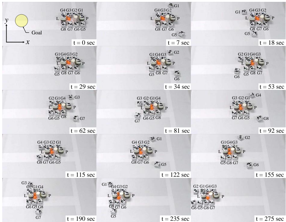
Figure 6.6 Multi-object transportation with a straight path. Three objects, including rolling objects, were transported successfully in 275 seconds.
