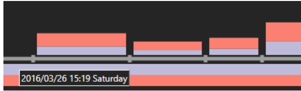
Figure 22. The tick marks can be dragged, added, and removed in order to adjust the interval of date-time range.
