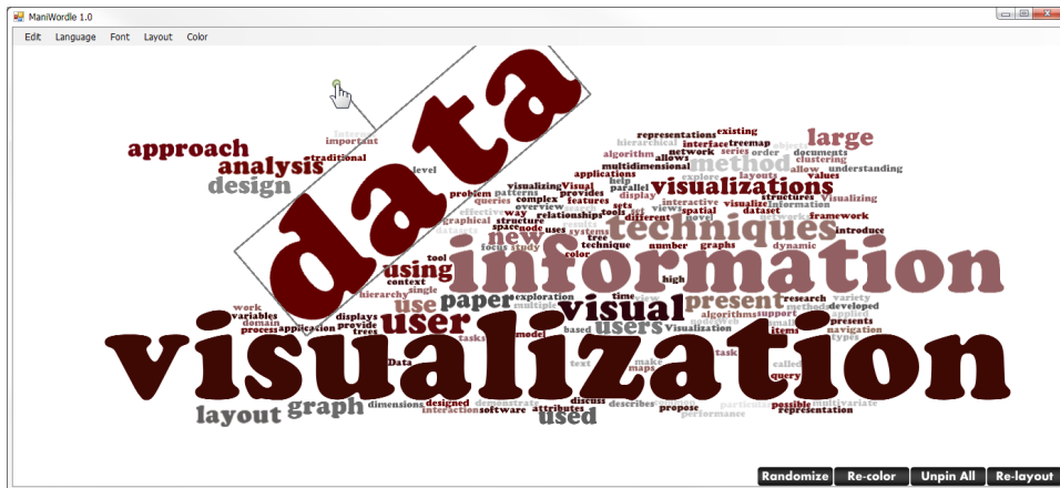
Figure 8. Main overview of ManiWordle showing a word cloud for the title and abstracts of All InfoVis Papers published since 1995. The word ‘data’ is selected and being rotated by dragging the circular handle on top.
