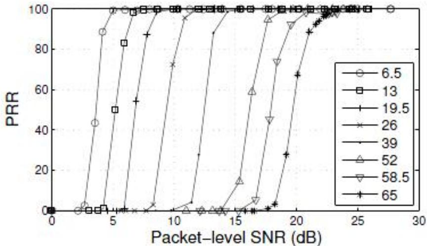
**Figure 5: Predictable relationship between SNR and packet reception rate (PRR) for flat fading link**
