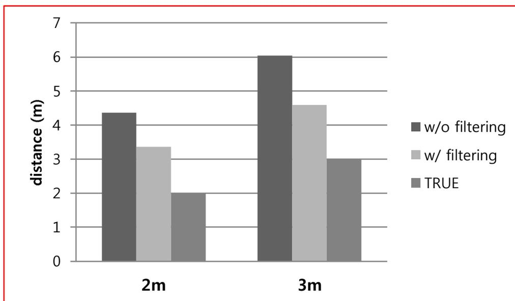
**Figure 9: Distance estimation before and after filtering**
