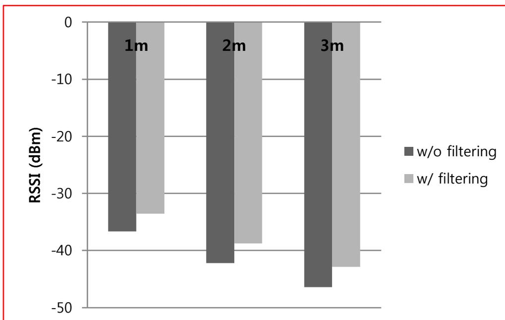
**Figure 8: RSSI before and after filtering**
