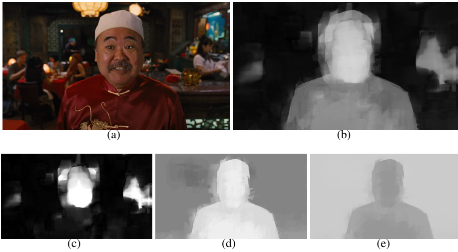
Figure 2.7: Result images for test sequence 1. (a) Test frame's left image. (b) VAP map. (c) V map. (d) DFS map. (e) DBA map. White represents a big value.
