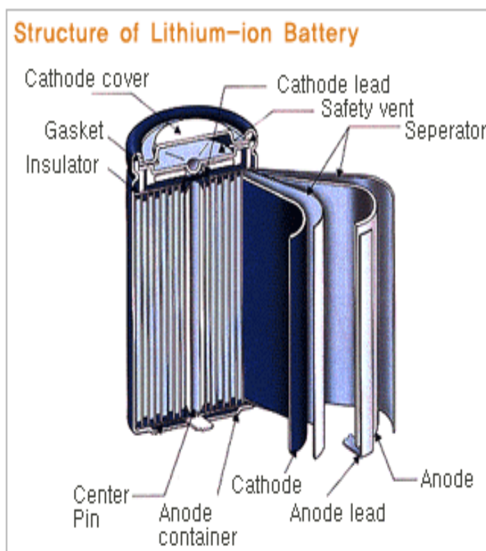
Figure 1.2 Structure of Lithium-ion battery in commercial production.
