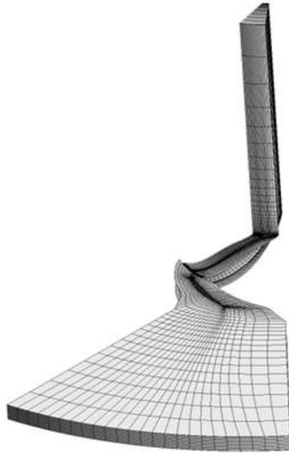
Fig. 2.3 Grid for single passage of the compressor.
