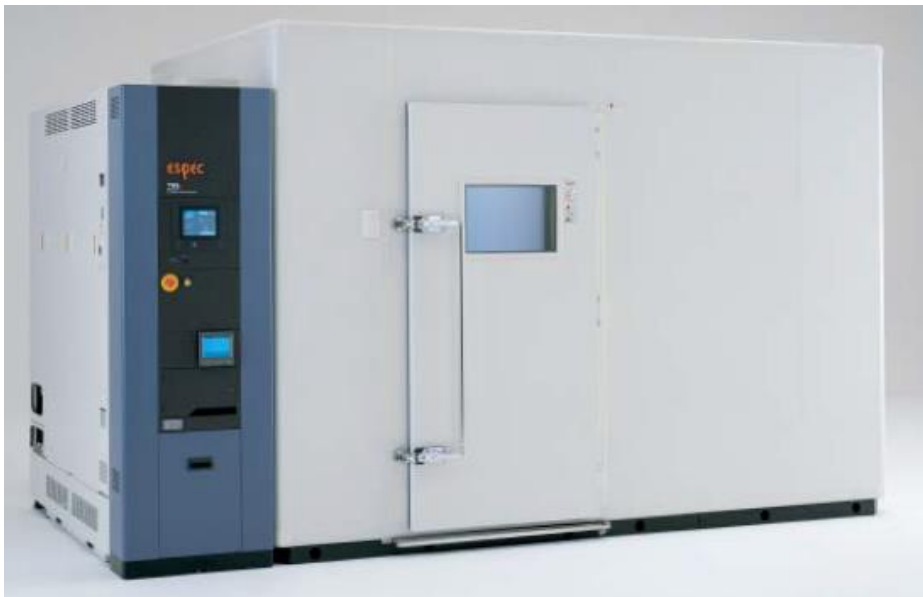
Figure 3.2 Picture of the constant temperature and humidity chamber
