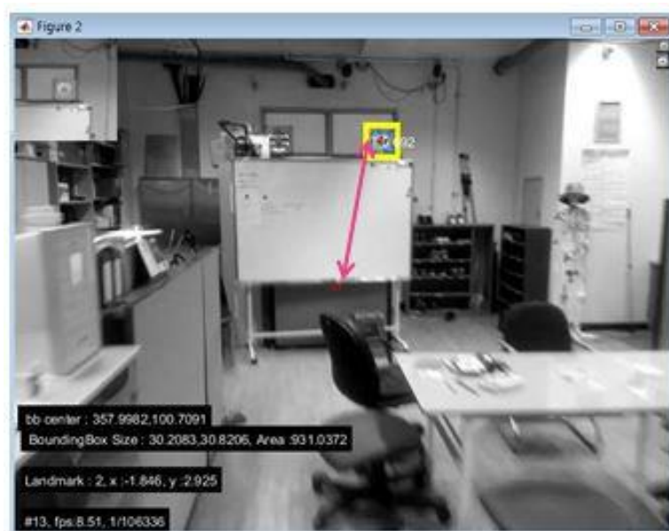
Figure 6. Landmark Selection from camera using TLD tracker. The linked information of landmarks is shown and the distance between the bounding box and the principal point is represented.
