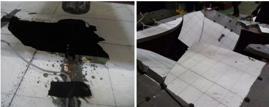
(a) d = 40\text{mm}, \rho_f = 0.0\% (Right after the loading : Left, After removal of jig : Right)
