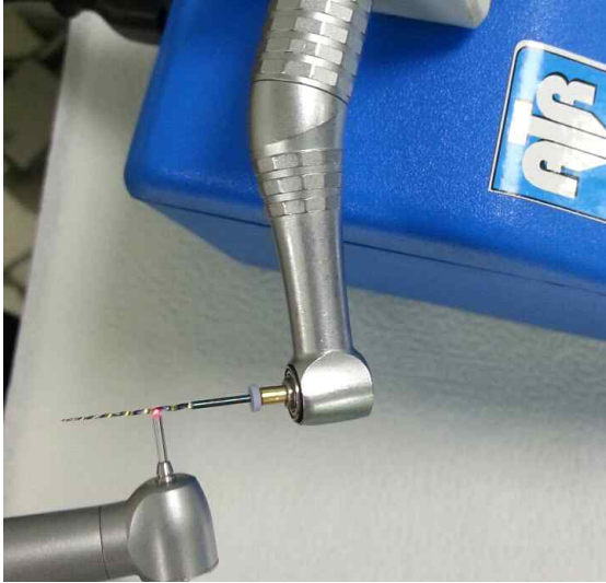
Figure 1. NiTi surface laser treatment of Group L
