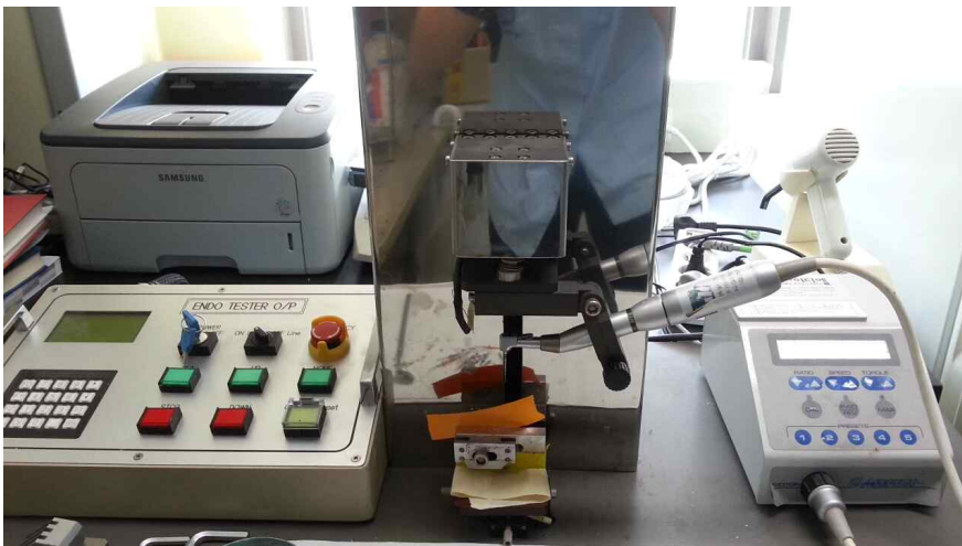
Figure 2. Cyclic fatigue test simulator
