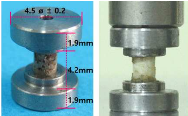
Fig 4) Compression yield strength measurements (0.2% offset), 1 mm/min compression.
