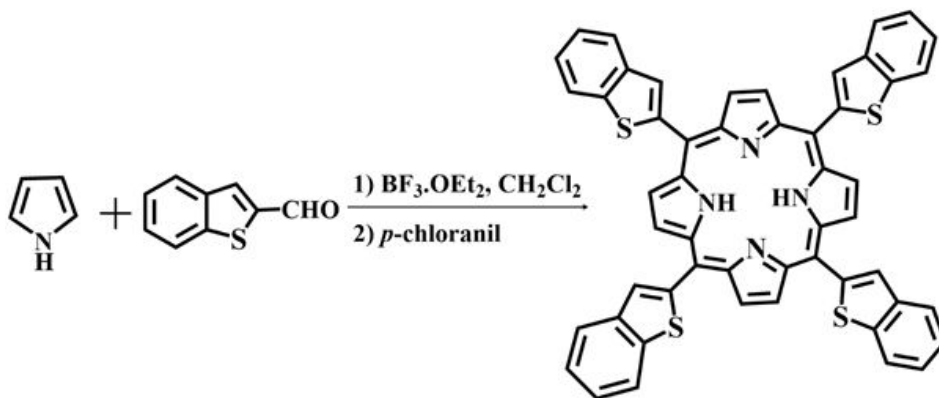
Figure 1. The reaction scheme of the synthesis for 5,10,15,20-tetrakis-(benzo[b]thiophene)porphyrin
