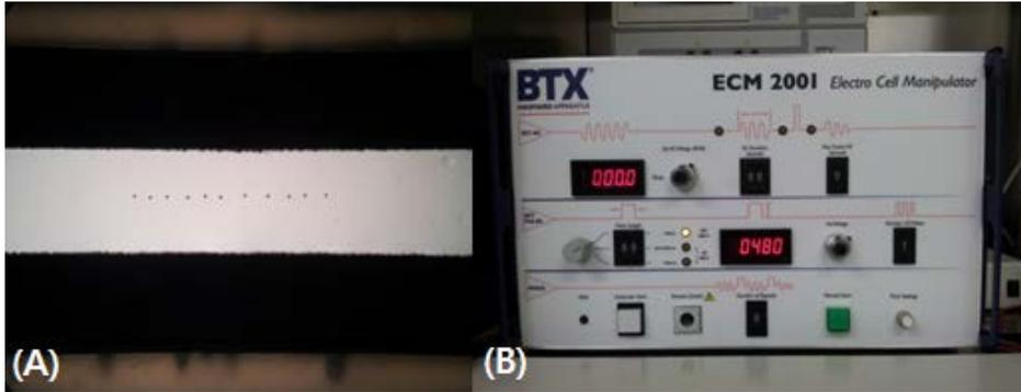
**Figure 3. Parthenogenetic activation by electrical stimulation.** Denuded oocytes were arranged in a row between two electrodes in a chamber which apart 3.2 mm (A) and filled with activation medium. Influx of  $\text{Ca}^{2+}$  into the oocytes was induced using a BTX electro-cell Manipulator (B).
