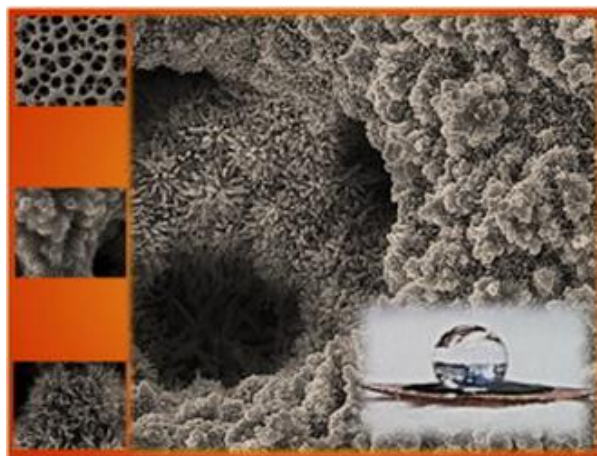
Figure 4. FE-SEM image of porous copper electrodeposited on to copper foil and contact angle.
