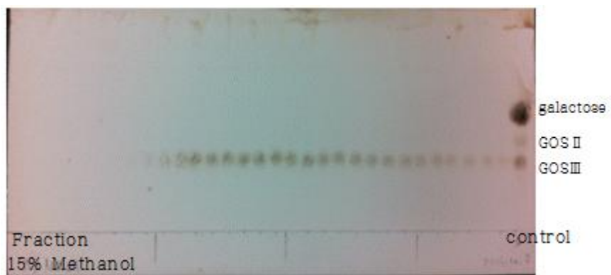
Fig. 5 The result of GOSIII purified by SPE was analyzed by TLC.
