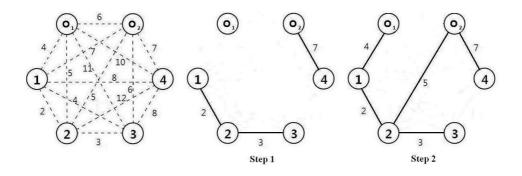
Figure 1: A 2s-mcstp and its mcst following the Boruvka algorithm
