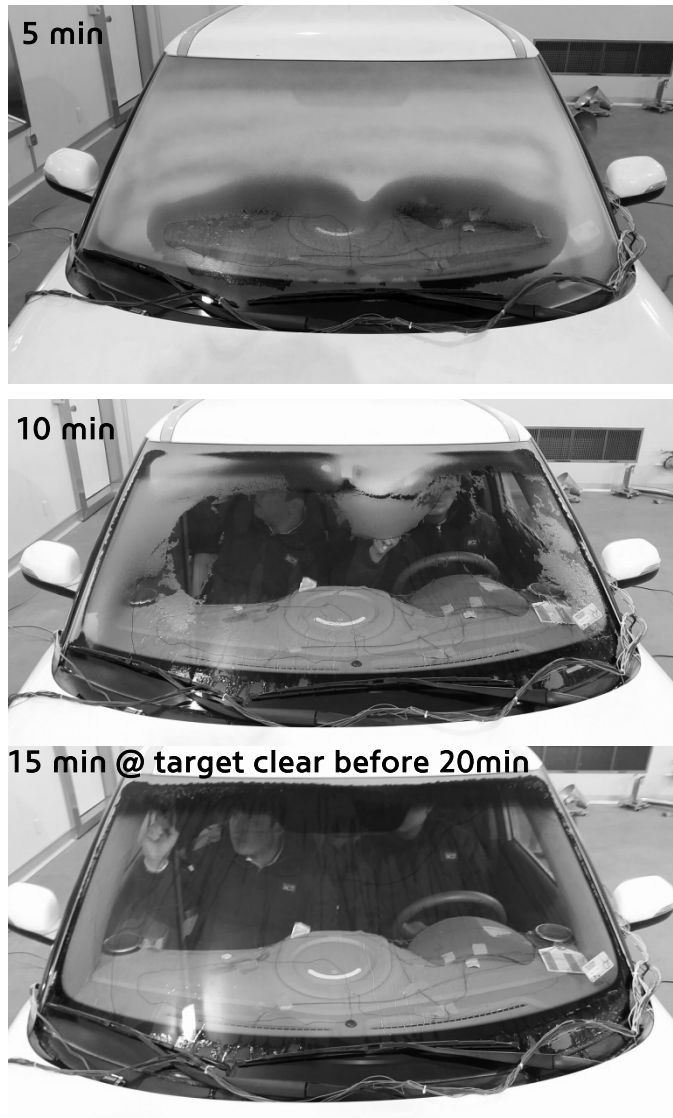
Figure 4.6 Windshield glass defrosting performance with CCHP for regulation
