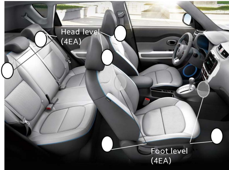
Figure 4.2 Positions for cabin temperature measurement
