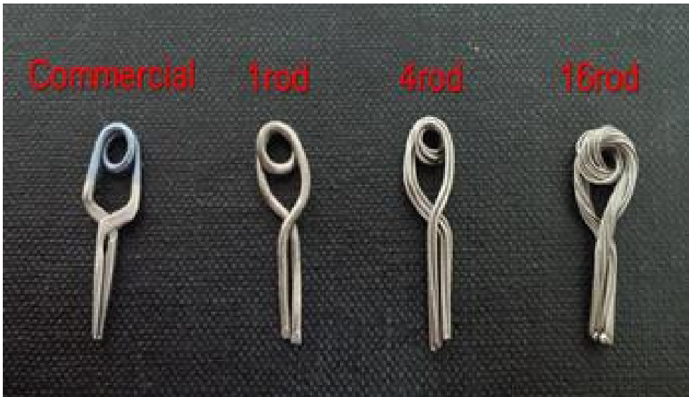
Figure 1. Titanium clips made from lamellar cylinder bundles
