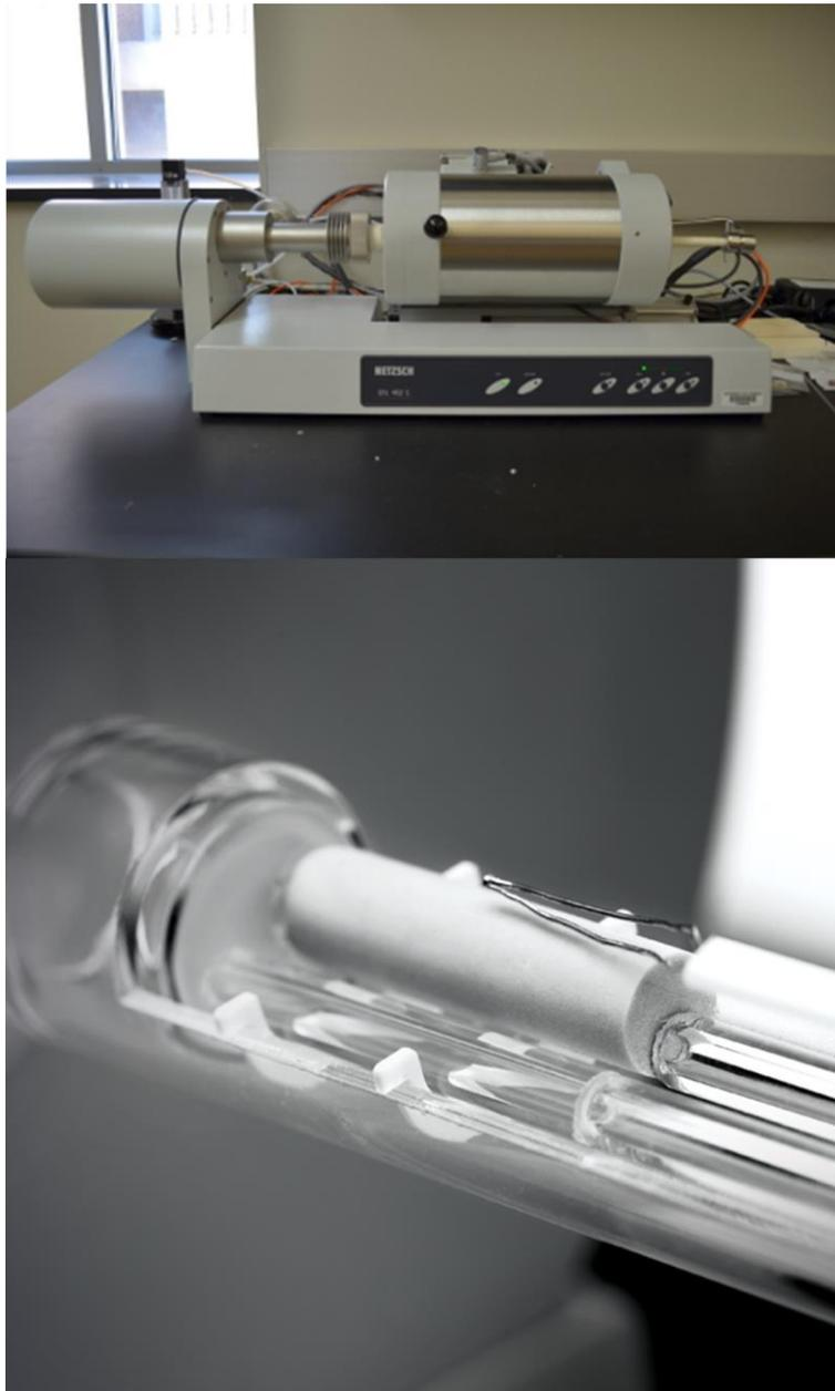
**Fig. 2.8.** Overview and loading stage of dilatometer for measuring volume change during martensitic transformation
