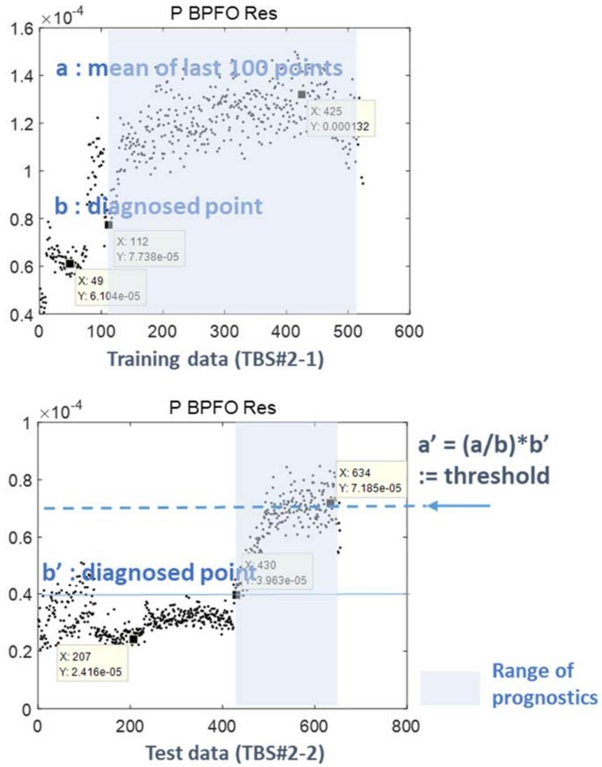
Figure 2-10 Ratio-based threshold decision method
