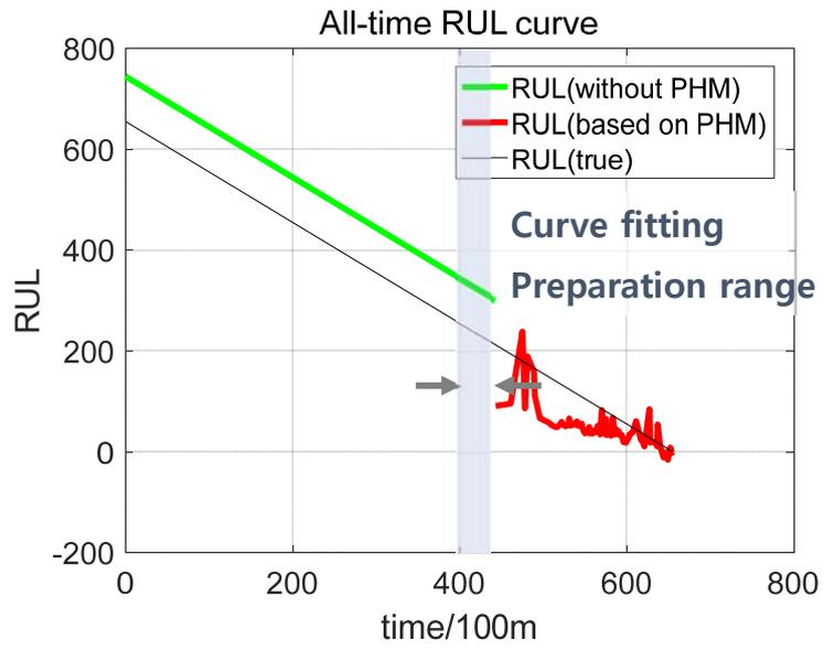
Figure 3-2 Full-time RUL curve with fading fatigue life  $L_{10}$
