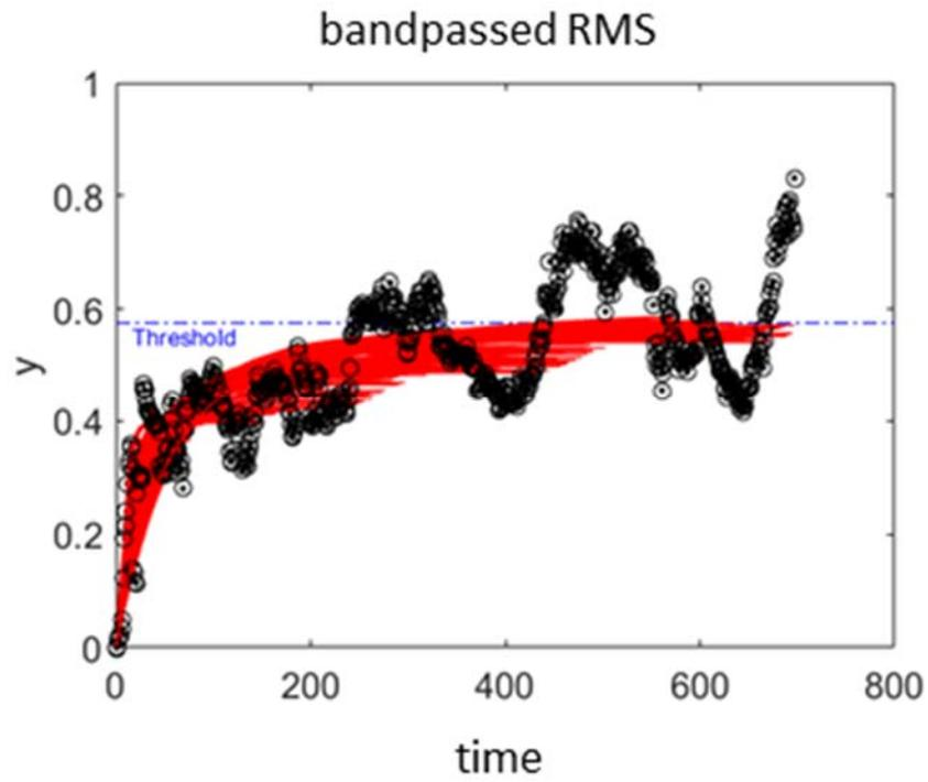
Figure 4–10 Bandpass–filtered RMS feature trend and projected curves of Normal #14 with threshold from Normal #13 data
