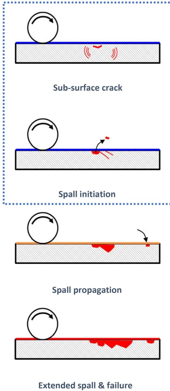
**Figure 2–7** Stages of rolling contact fatigue and degradation
