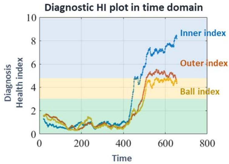
Figure 2–8 Fault diagnosis plot for inner race, outer race, and ball
