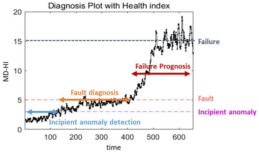
Figure 2–5 Bound definition of incipient anomaly and fault based on MD
