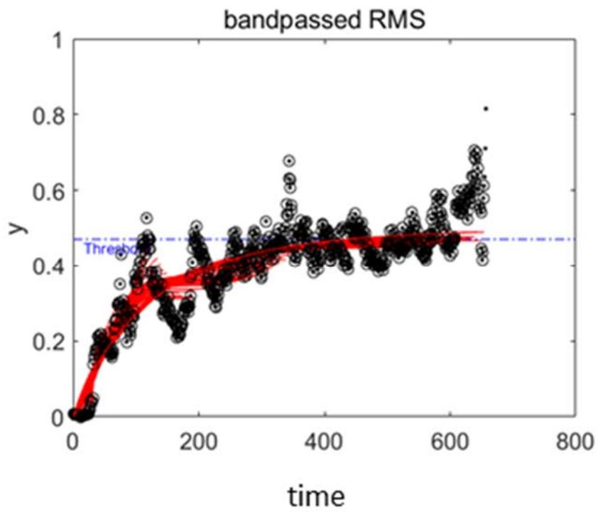
Figure 4-6 Bandpass-filtered RMS feature trend and projected curves of Normal #17 with threshold from Normal #12 data
