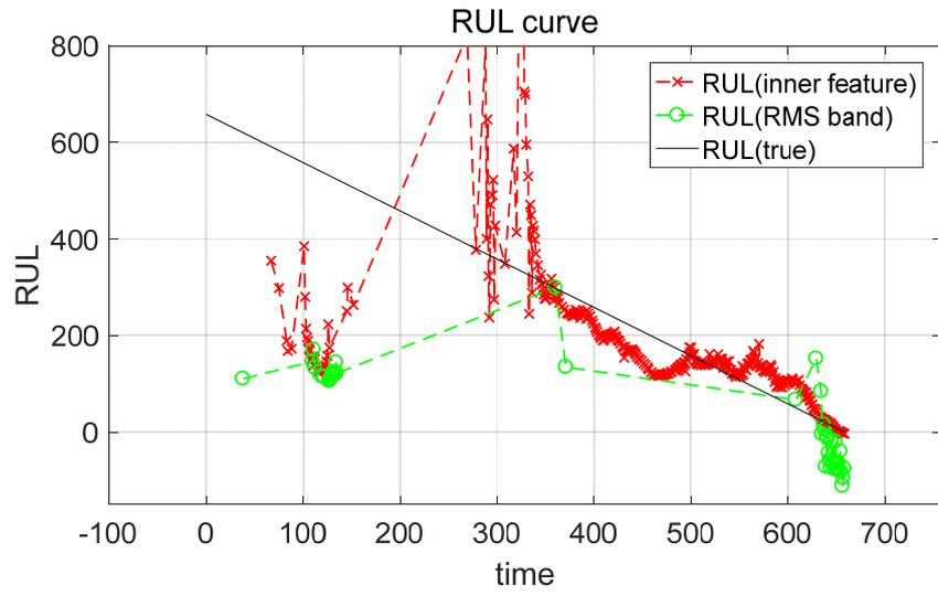
Figure 4-3 RUL prediction result with inner race feature and bandpassed RMS feature
