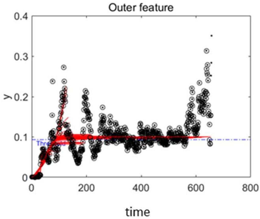
Figure 4-5 Outer race feature trend and projected curves of Normal #17 with threshold from Normal #12 data
