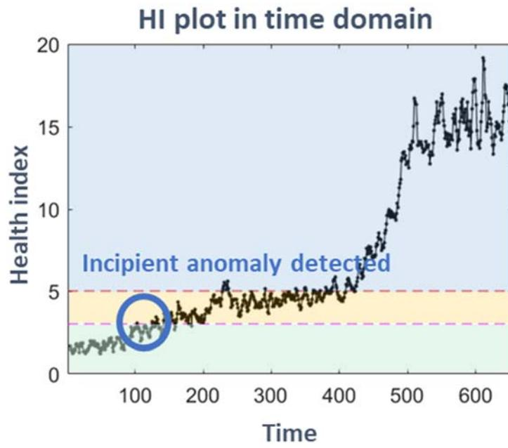
Figure 2–6 Results of incipient anomaly detection
