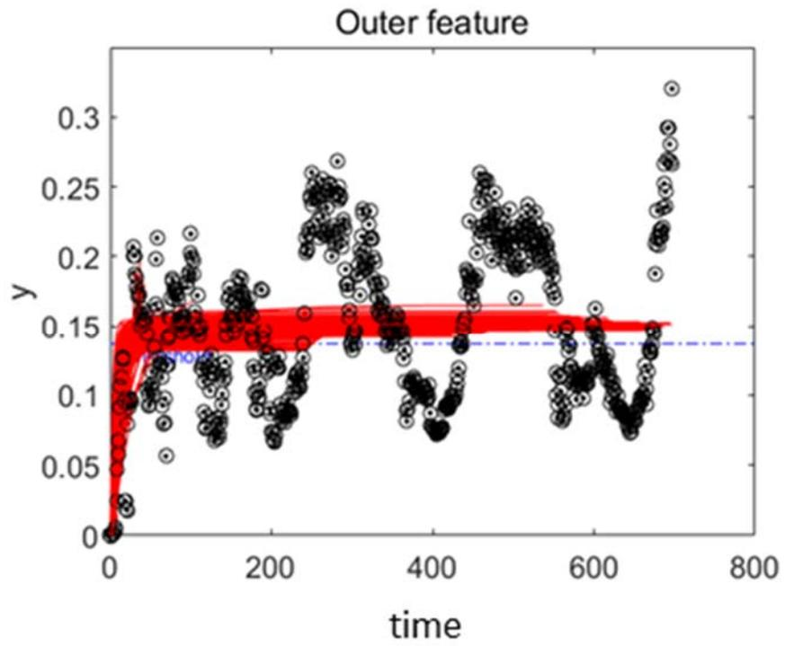
Figure 4-9 Outer race feature trend and projected curves of Normal #14 with threshold from Normal #13 data
