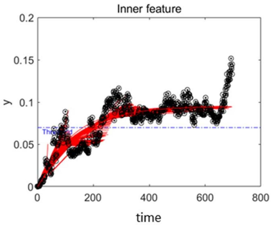
Figure 4-8 Inner race feature trend and projected curves of Normal #14 with threshold from Normal #13 data
