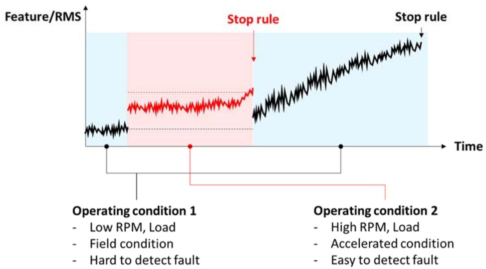
Figure 4–2 SNU bearing test sequence
