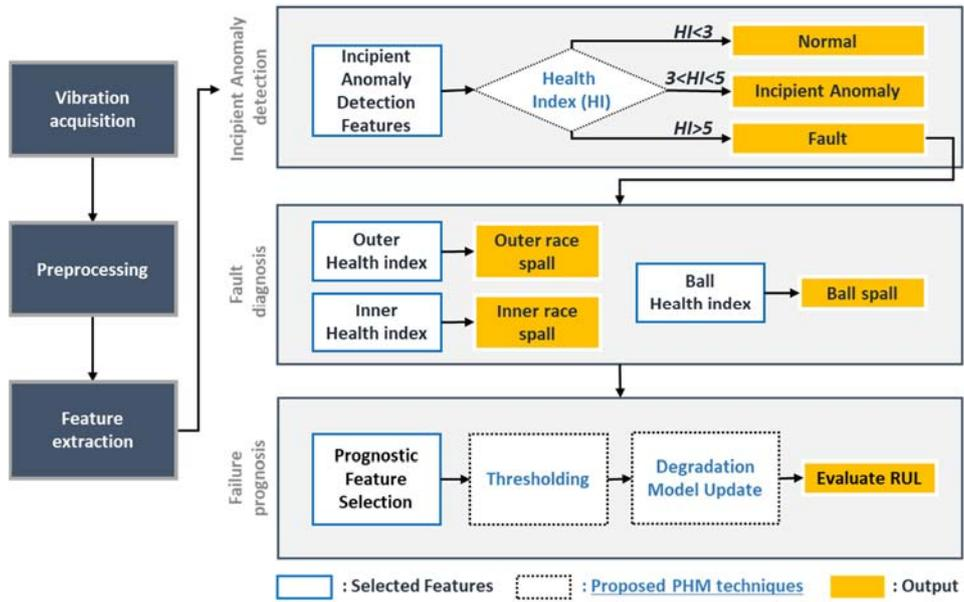
Figure 2-1 PHM flowchart for health monitoring of bearings
