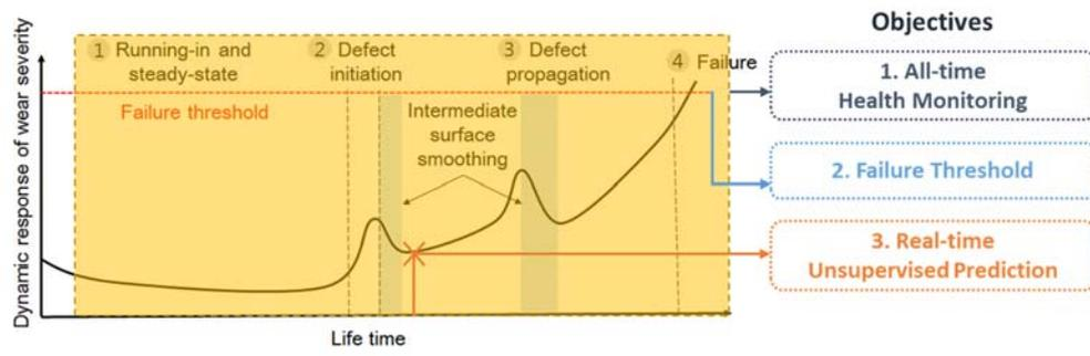
Figure 1–1 Research objectives throughout the life of a bearing
