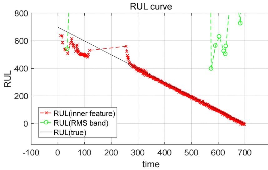
Figure 4-7 RUL prediction result with inner race feature and bandpassed RMS feature (Normal #13, 14)
