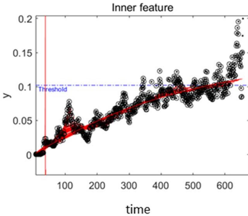
Figure 4-4 Inner race feature trend and projected curves of Normal #17 with threshold from Normal #12 data
