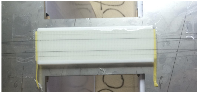
Figure 3.1 Scaffold, SMA wires and regular wires encased in PDMS
