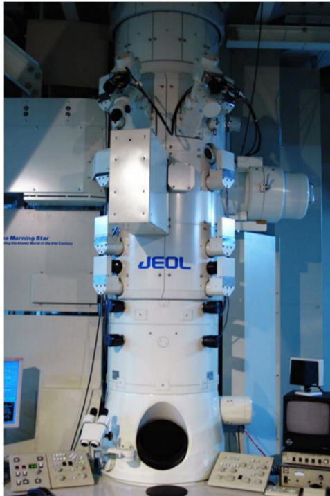
Figure 2.9 TEM instrument of ARM 1300S in KBSI for electron irradiation [29].
