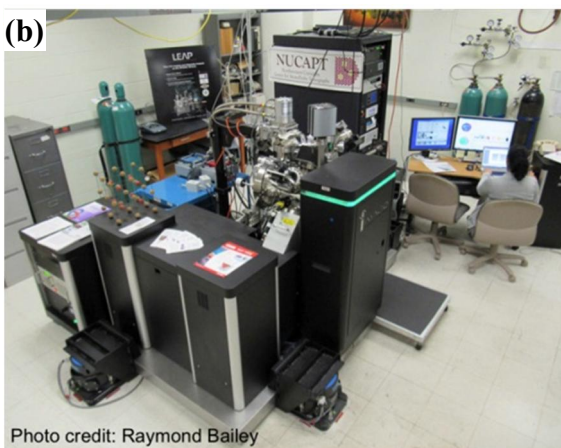
Figure 2.6 APT instruments of (a) LEAP 4000X HR in KIST and (b) LEAP 4000X Si in Northwestern University.
